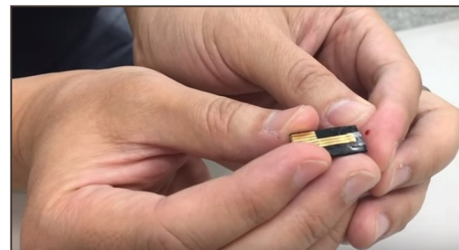
The portable biosensor can test specific cardiac markers in five minutes with a single drop of blood.
